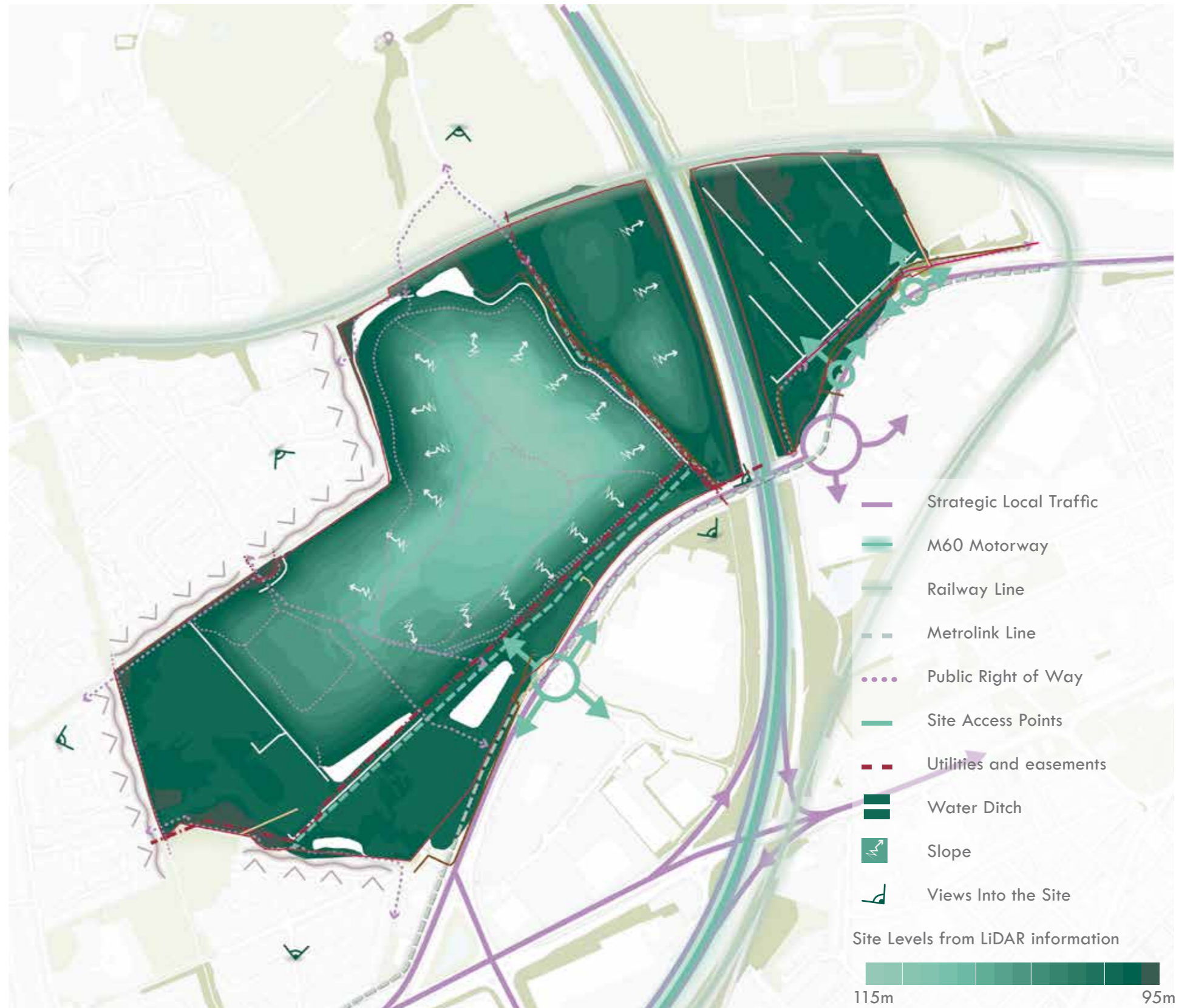
Figure 4.2: Existing general site wide levels
